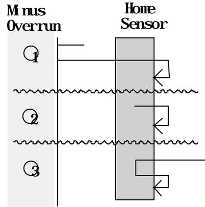
**6-2-1-2: Home Mechanism for Motor with Encoder**
